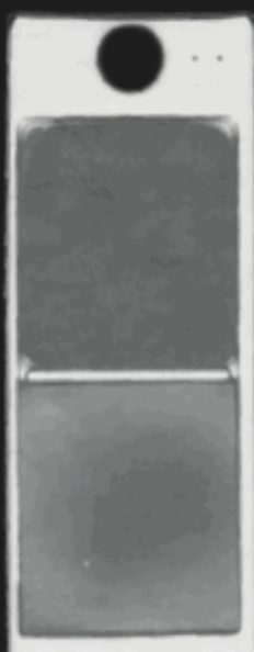
Figure 4. Ultrasonic scanning of the MIFA module's soldered joint
