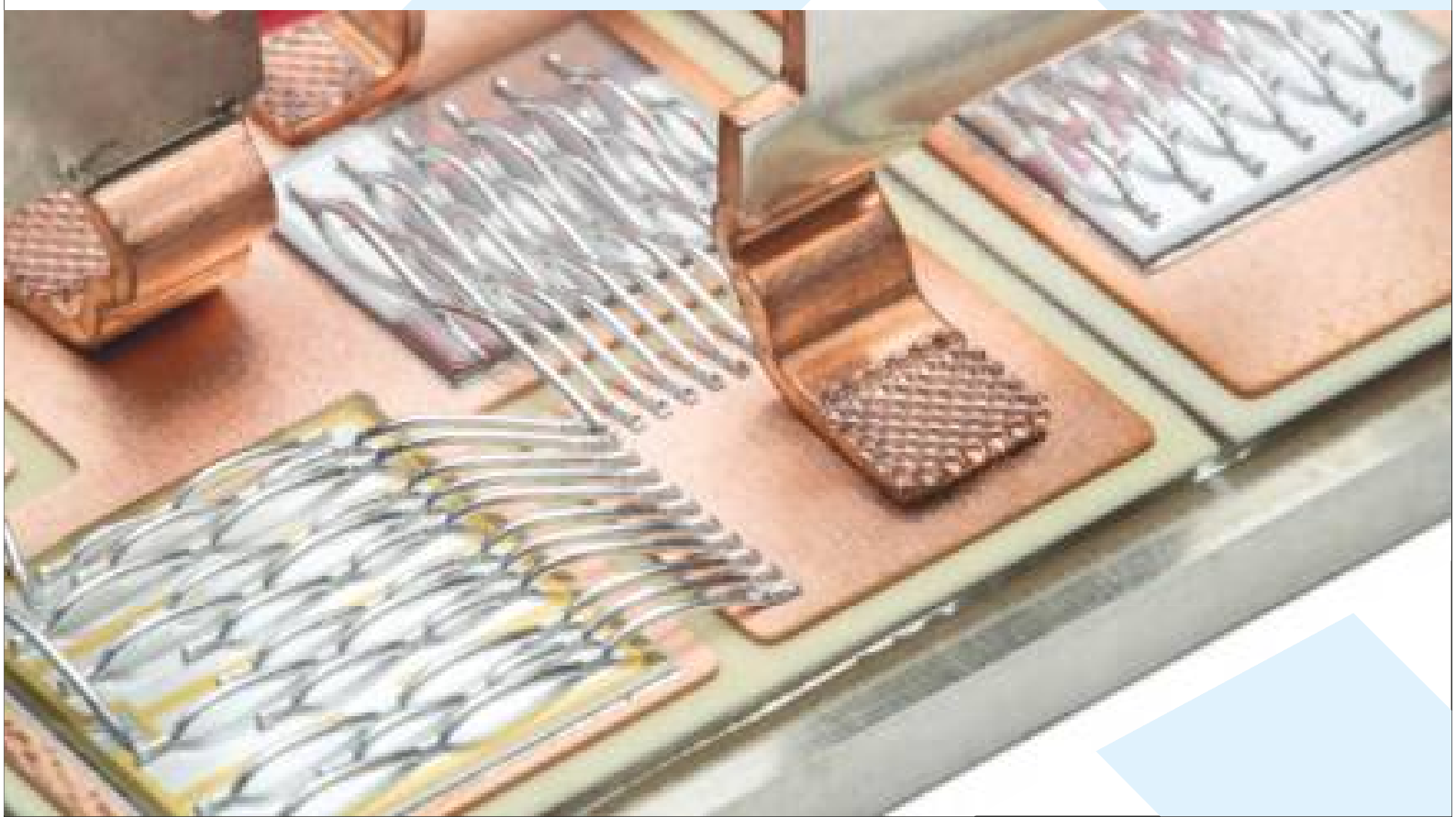
Figure 5. Ultrasonic welding of power leads
